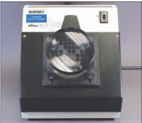
2.3 Colony Counter ■ Subtle differences in colony shape and size can best be viewed with magnification, such as is provided by a colony counter. The transmitted light and magnifying glass allow observation of greater detail; however, colony color and many other features are best determined with reflected light. The grid in the background is a counting aid; each big square is 1 square centimeter.
